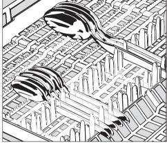
Spoon heads should be placed so that water can run off freely.
